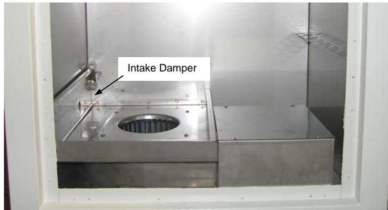
CONDITIONING PLENUM – INTAKE DAMPER FULLY CLOSED
