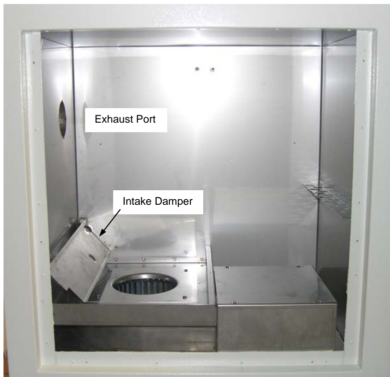
CONDITIONING PLENUM – INTAKE DAMPER FULLY OPEN
