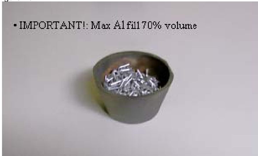
Properly filled Graphite liner with Al
