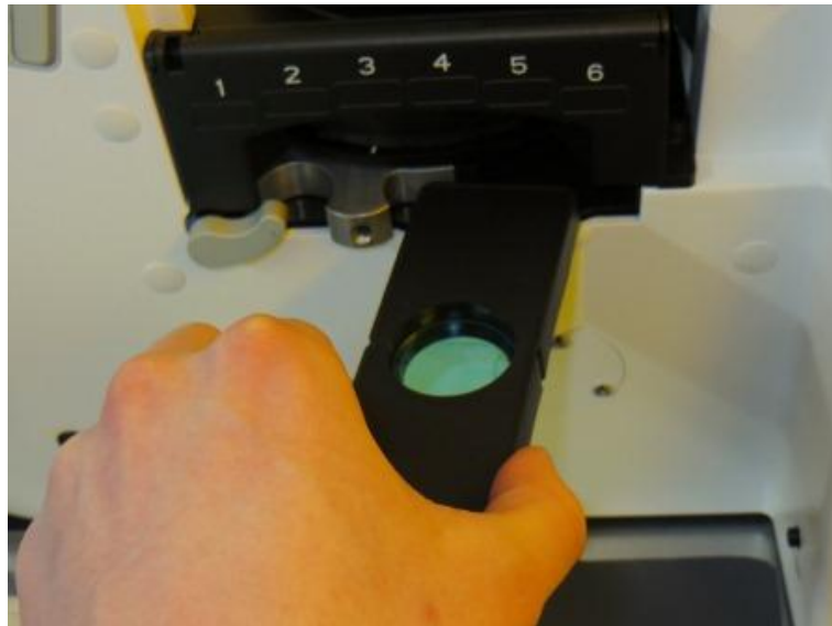
Figure A.6.: Removing the green filter which is located next to the reflector turret handle.
