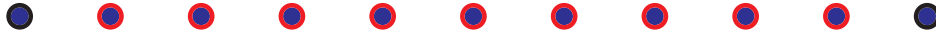
Figure 7.20.: Illustration of the coded coordinates (black circles), the automatically added coordinates (red circles) and the written result (blue dots) in PulsedMode and with ConnectPointsOn .
