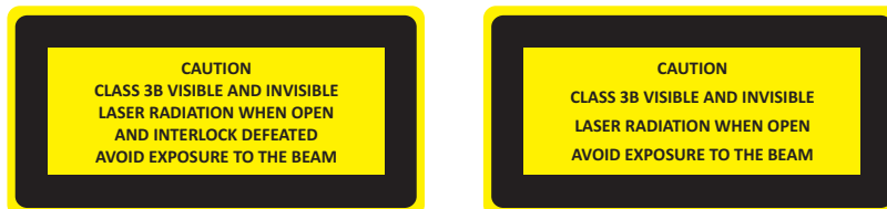
Figure 2.3.: The two types of laser warning labels are attached to the system
