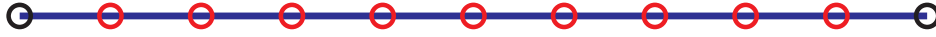
Figure 7.18.: Illustration of the coded coordinates (black circles), the automatically interpolated coordinates (red circles) and the written result (blue line) in ContinuousMode and with ConnectPointsOn .
