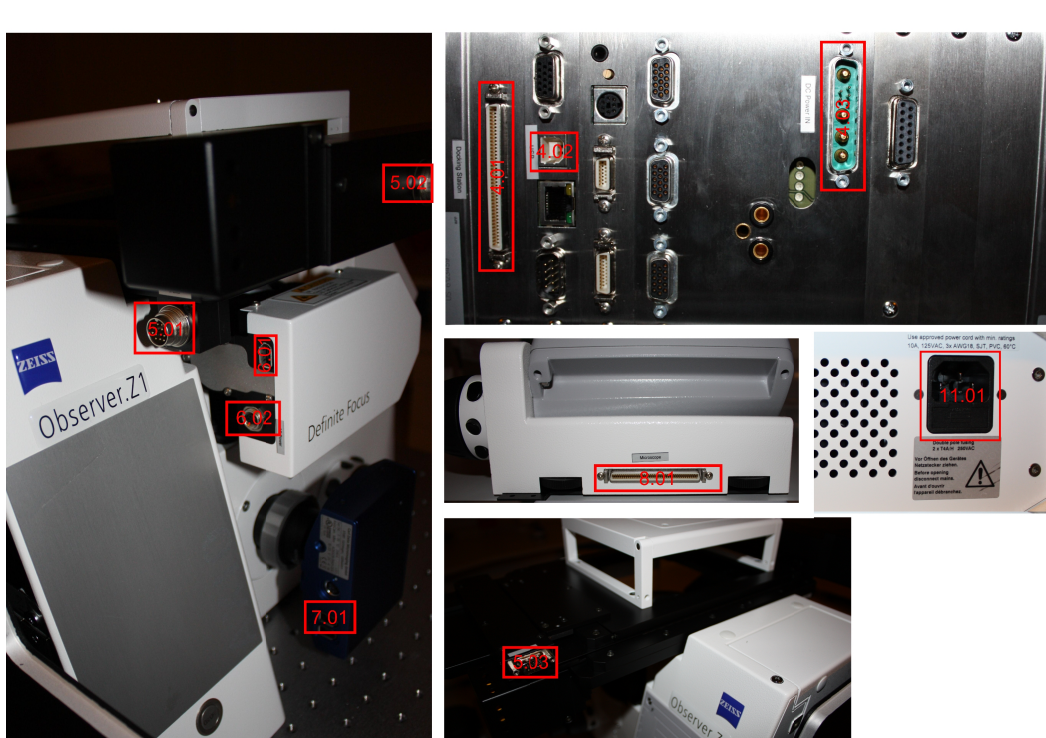
Figure 2.9.: Autofocus (6.), live camera (7.), motorized stage (5.), microscope backpanel (4.), microscope docking station (8.) and microscope power supply (11.)
