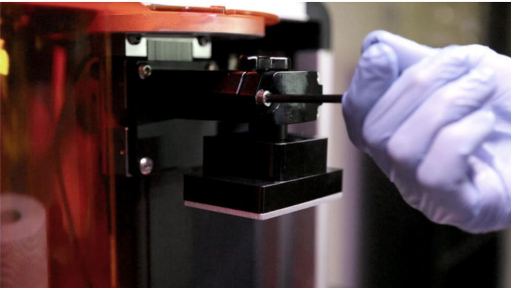
We'll need to relevel the build head before starting a new job - mainly because it misaligns after removal. So we can loosen the build plate and move it up, and then we'll tighten up the screw.
