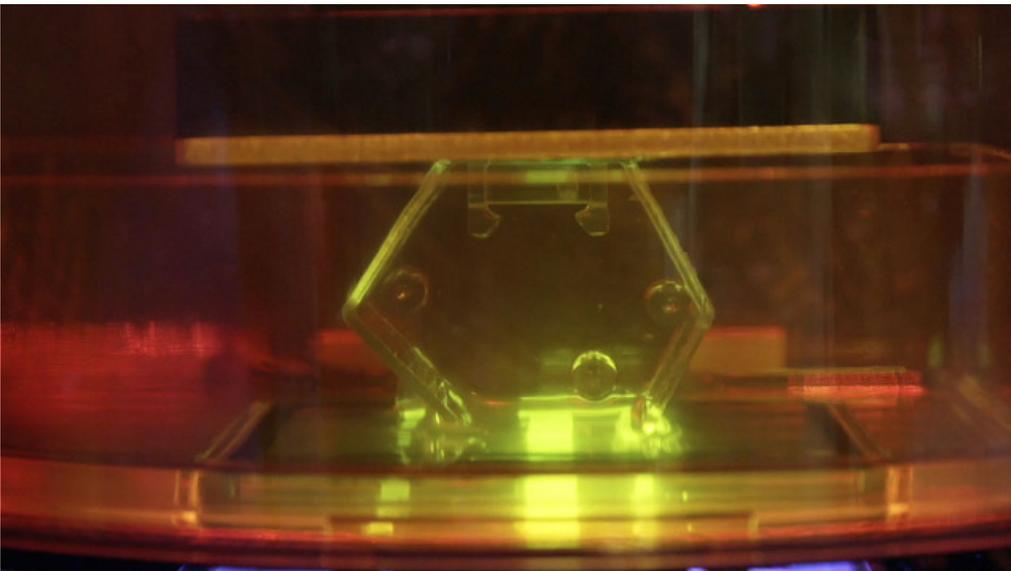
The ember printer uses a cure and peel technique. This exposes and separates for each layer to create a high definition part.
