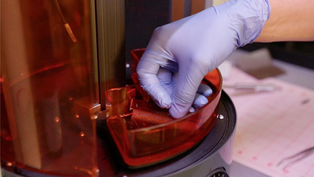
Keeping the resin tank clean is important. As prints fail, material builds up and floats around the tray. These can be difficult to spot, so we can use a hair comb to filter out any pieces left behind. Use tweezers to fetch out any bigger pieces.
